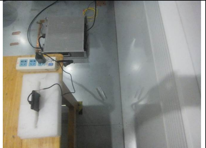
Conducted Emissions Test Setup Side View
