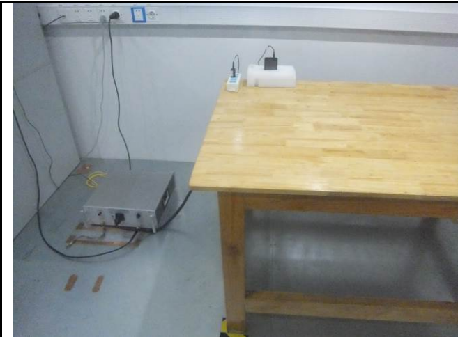
Conducted Emissions Test Setup Front View
