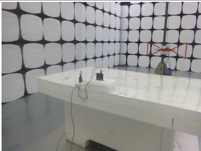
Conducted Emissions Test Setup Front View
