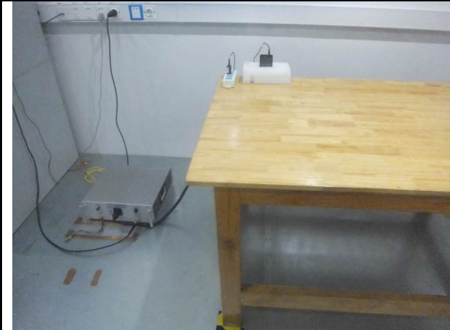
Conducted Emissions Test Setup Front View
