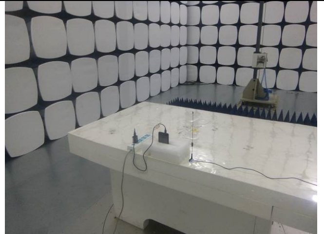
Radiated Spurious Emissions Test Setup Above 1GHz
