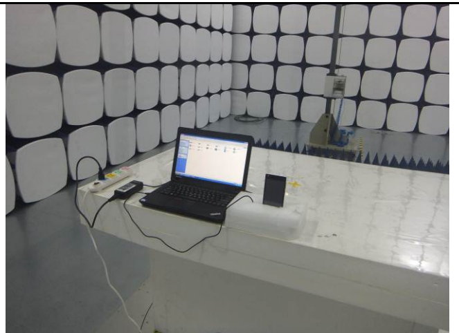
Radiated Spurious Emissions Test Setup Above 1GHz
