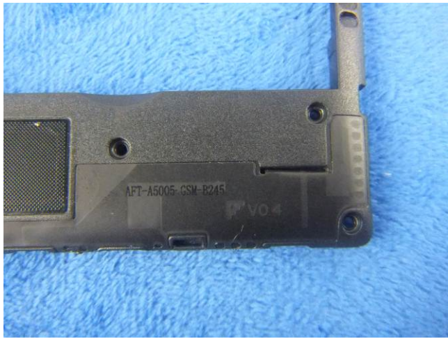
GSM/PCS/UMTS-FDD Antenna View
