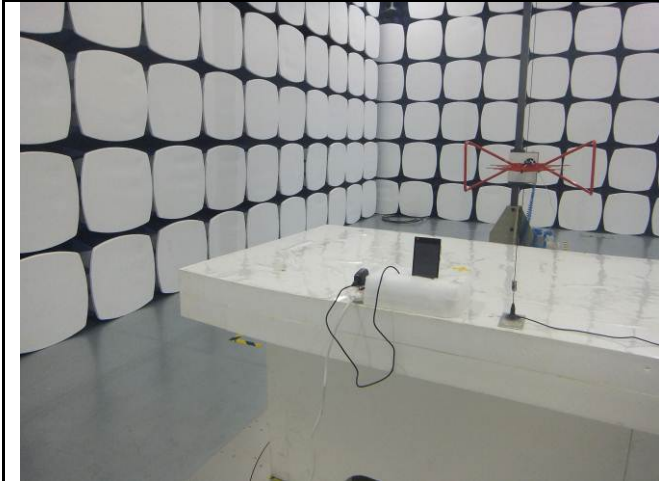
Radiated Spurious Emissions Test Setup Below 1GHz
