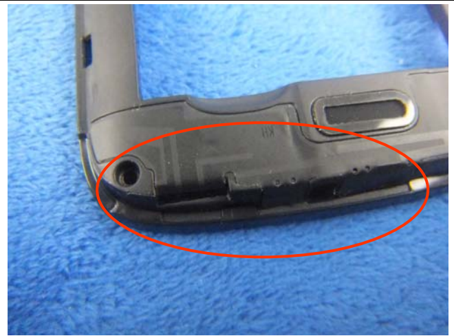
GSM/PCS/UMTS-FDD Antenna View
