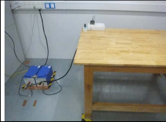
Conducted Emissions Test Setup Front View
