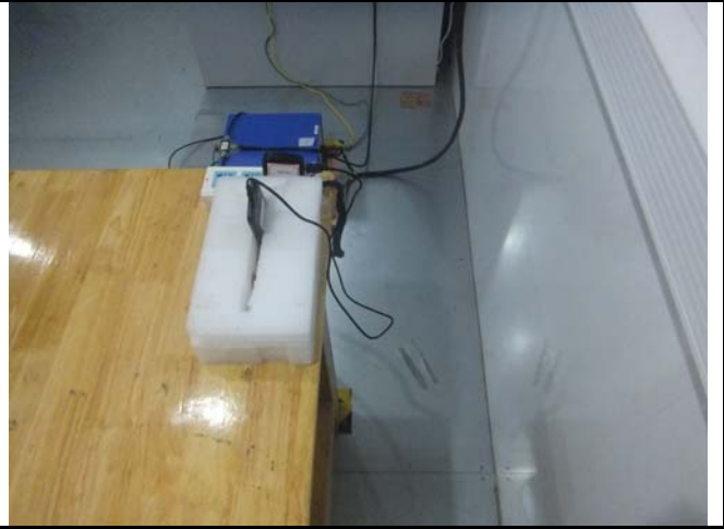
Conducted Emissions Test Setup Side View
