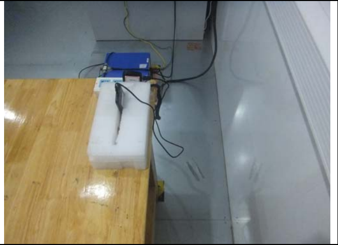
Conducted Emissions Test Setup Side View
