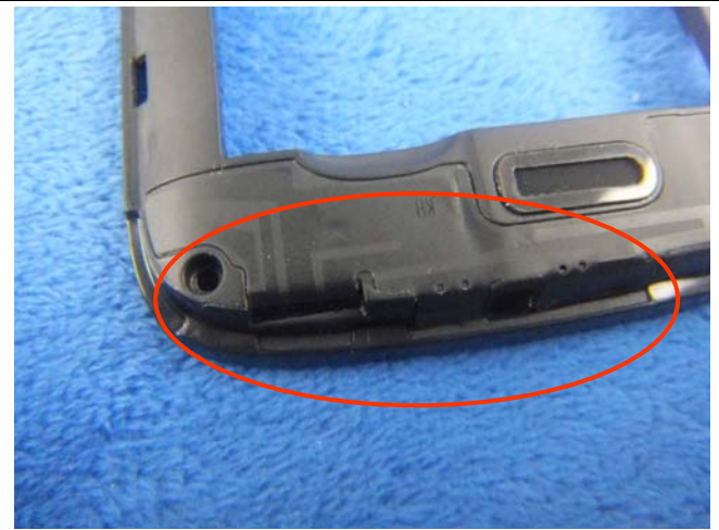
GSM/PCS/UMTS-FDD Antenna View
