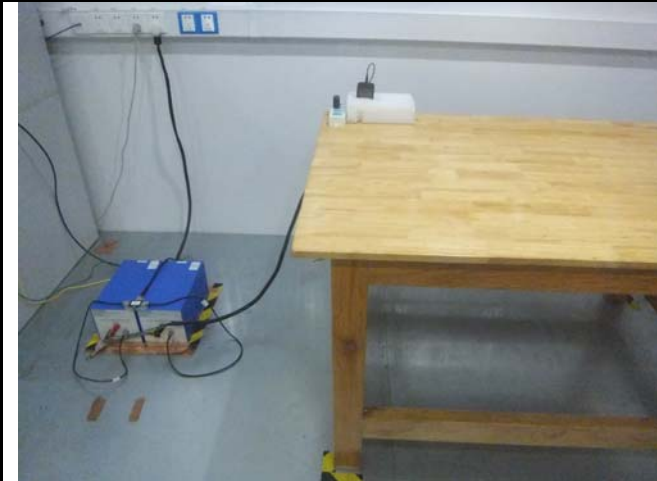
Conducted Emissions Test Setup Front View
