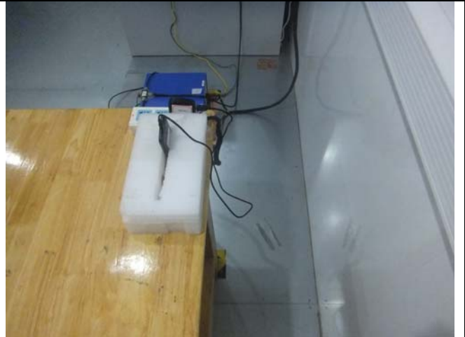
Conducted Emissions Test Setup Side View
