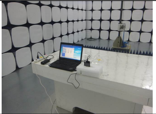
Radiated Spurious Emissions Test Setup Above 1GHz
