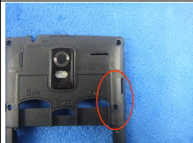
BT/WIFI Antenna View
