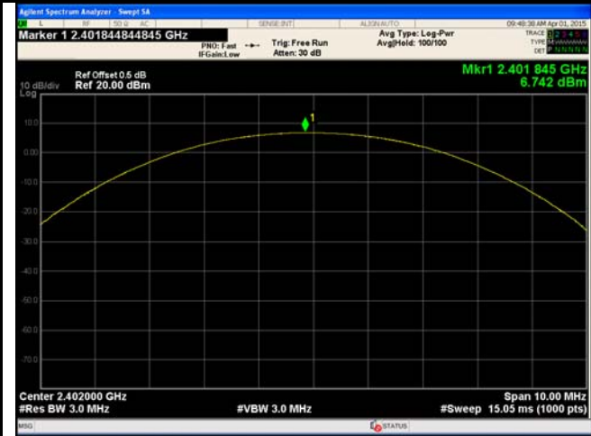
8DPSK Output power - Low CH 2402
