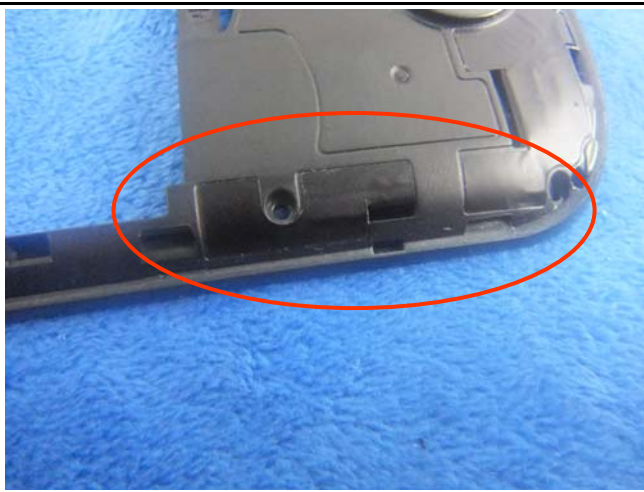
WIFI - Antenna View
