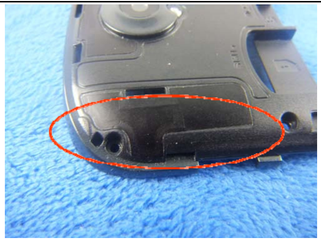
GSM Antenna View
