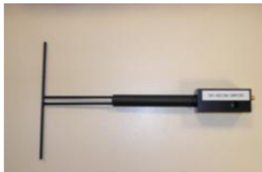
Figure 1 – Satimo COMOSAR Validation Dipole
