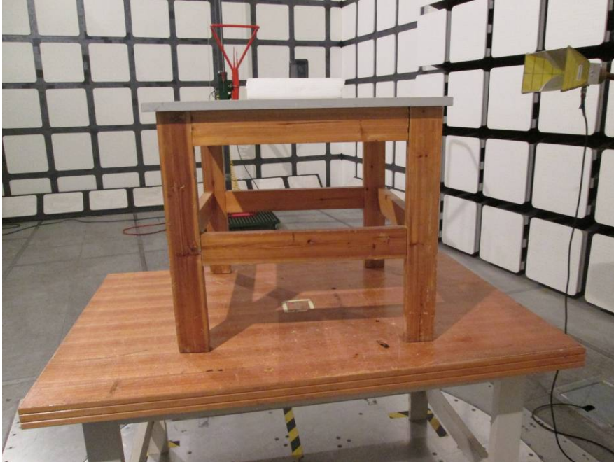
Radiated Emissions Test View (Below 1 GHz)
