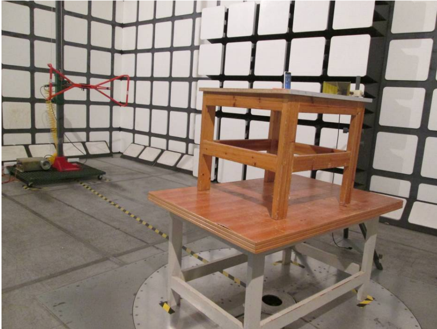
Radiated Emissions Test View (Below 1 GHz)
