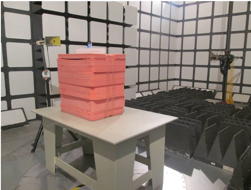
Radiated Emissions Test View (Above 1 GHz)
