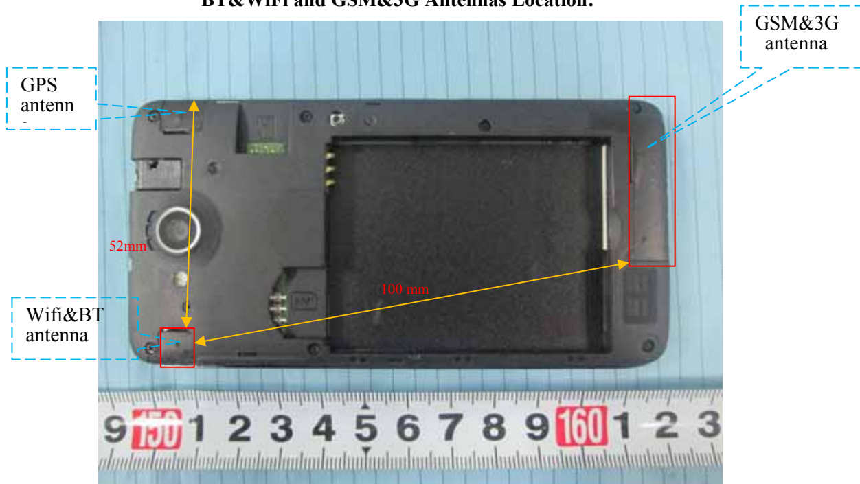
BT&WiFi and GSM&3G Antennas Location:
