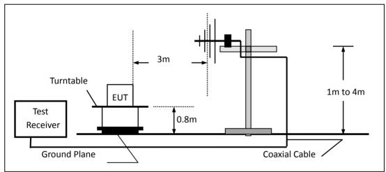
(c) For radiated emissions above 1000MHz
