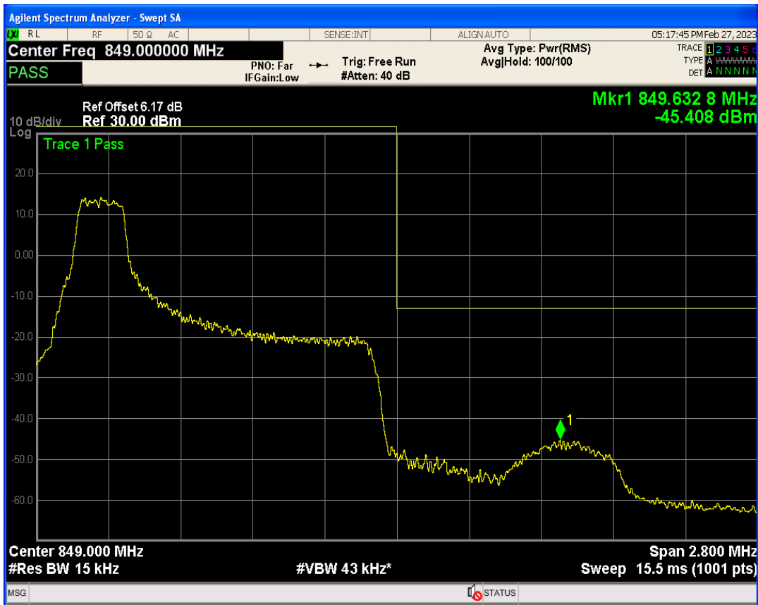
Band26b QAM16 BW=1.4MHz Channel=27033 RB Size=1 Position=#Max
