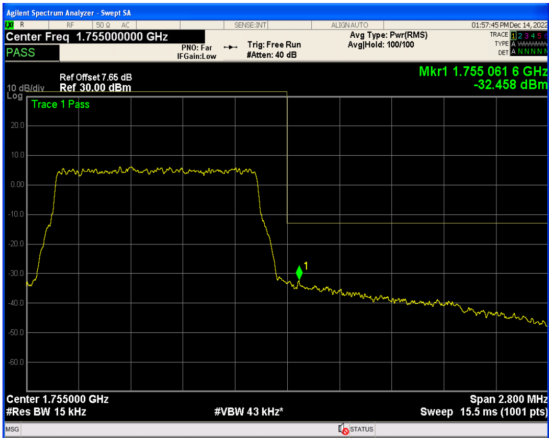
Band4 QPSK BW=3MHz Channel=19965 RB Size=1 Position=#0
