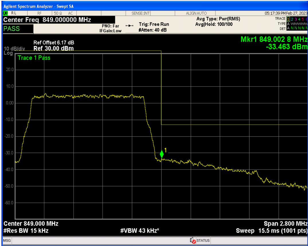
Band26b QAM16 BW=1.4MHz Channel=27033 RB Size=1 Position=#0
