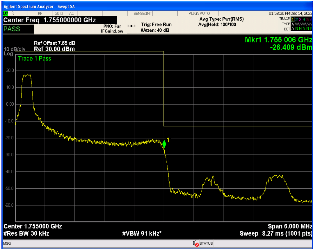
Band4 QPSK BW=3MHz Channel=20385 RB Size=15 Position=#0
