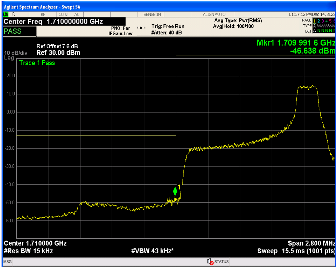
Band4 QPSK BW=1.4MHz Channel=20393 RB Size=1 Position=#0
