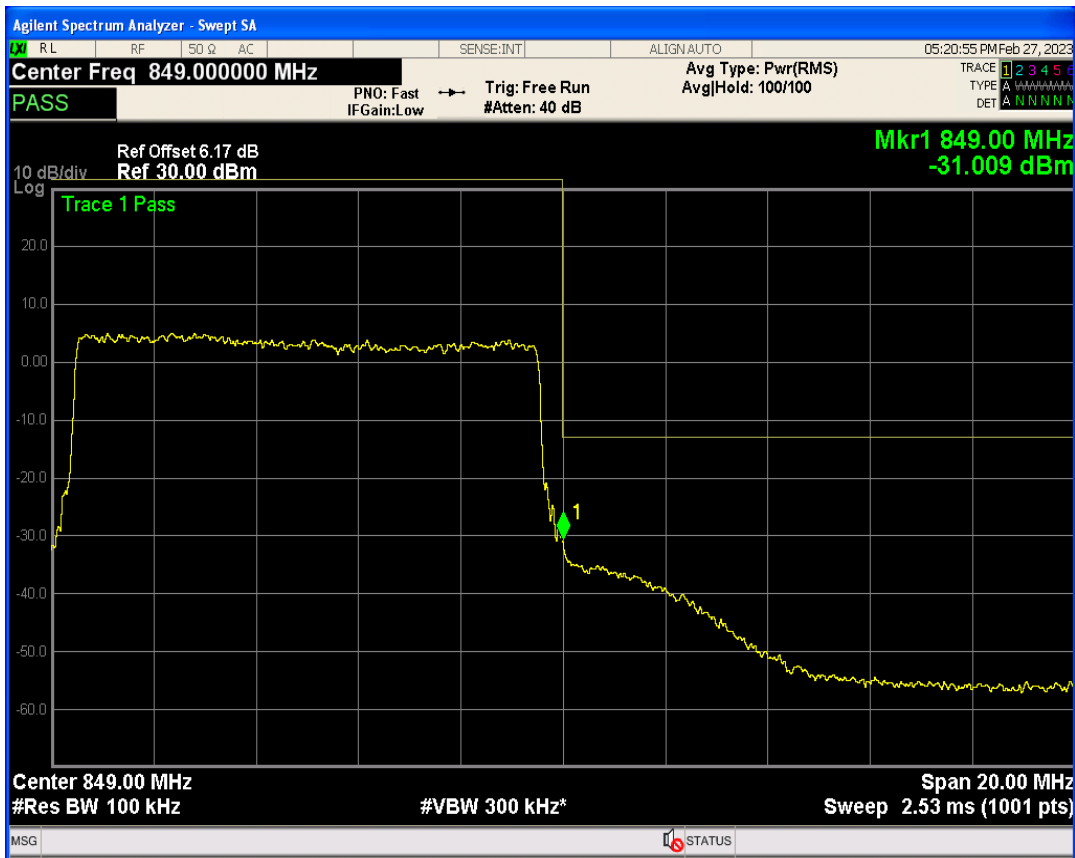
Band26b QAM16 BW=10MHz Channel=26990 RB Size=1 Position=#0
