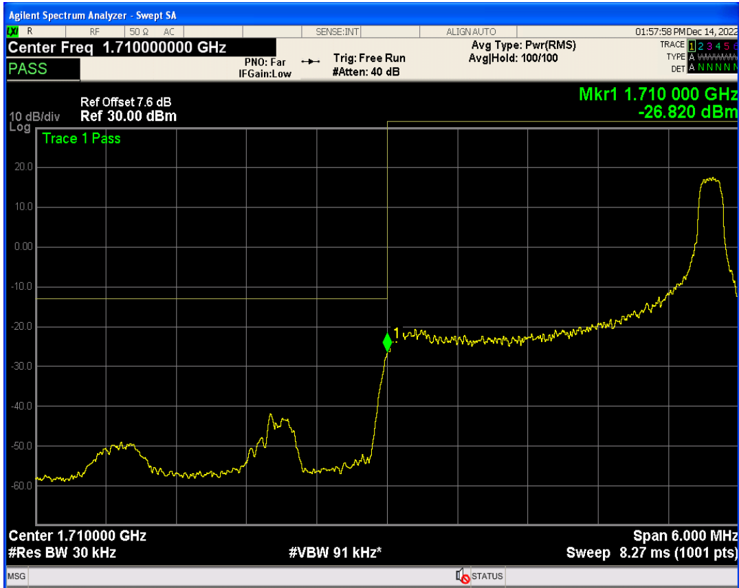
Band4 QAM16 BW=3MHz Channel=19965 RB Size=1 Position=#0
