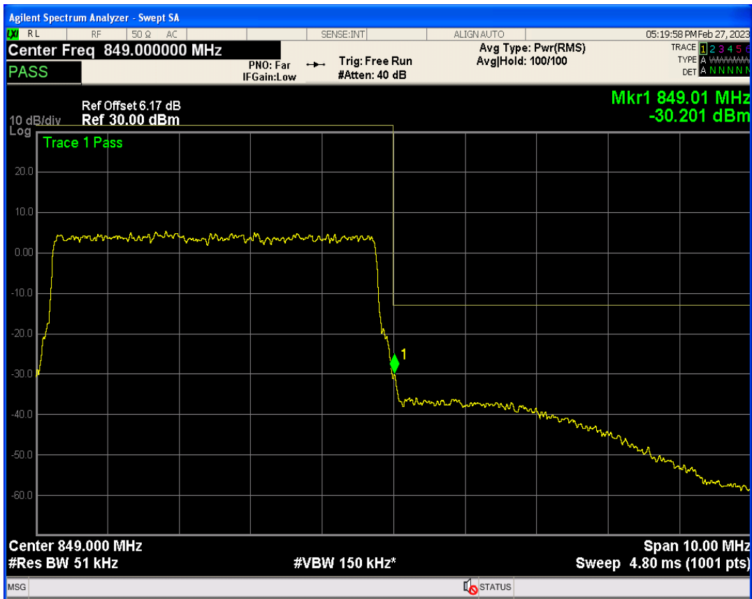
Band26b QPSK BW=5MHz Channel=27015 RB Size=1 Position=#Max
