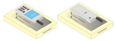
Picture 4 Test positions for body-worn devices
