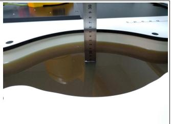
Liquid depth in the Head phantom
