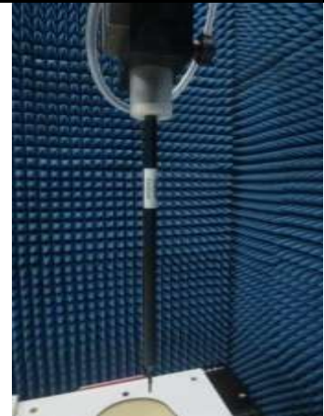
Fig.8.2 Photo of E-Field Probe
