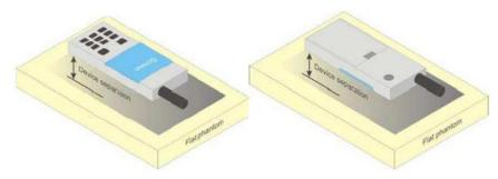
Picture 4 Test positions for body-worn devices
