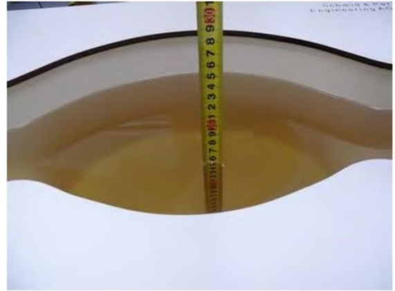
Liquid depth in the body phantom (835MHz)
