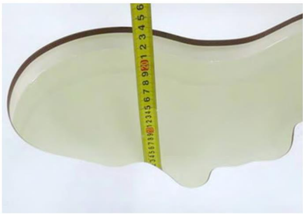
Liquid depth in the head phantom (1900MHz)
