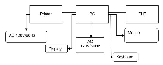
**Equipment Used in Tested System**
