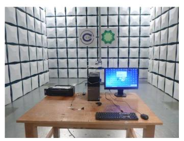
Radiated Emission (above 1GHz) Connect to PC
