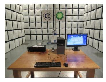
Radiated Emission (above 1GHz) Connect to PC
