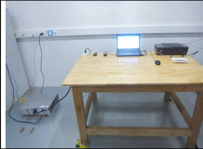
Conducted Emissions Test Setup – Front View
