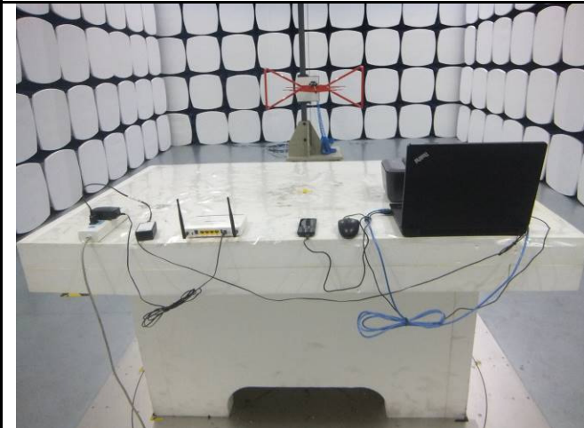
Radiated Emissions Test Setup Below 1GHz
