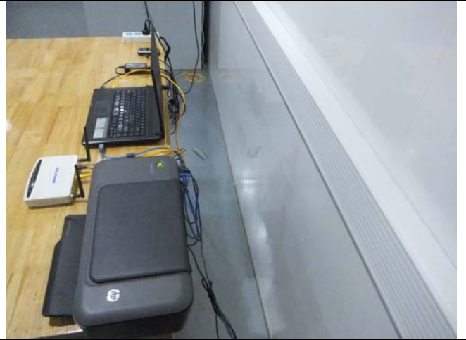
Conducted Emissions Test Setup – Side View
