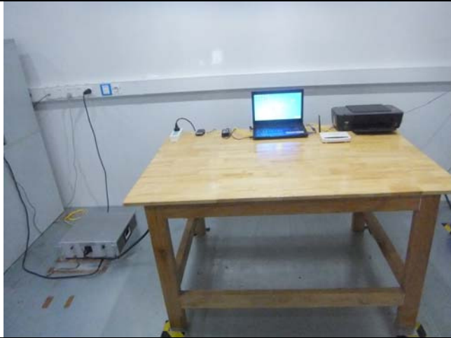
Conducted Emissions Test Setup – Front View
