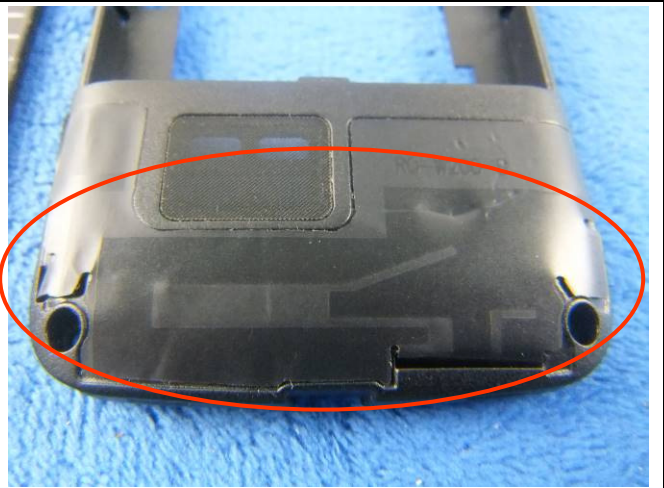
GSM/PCS/UMTS-FDD Antenna View
