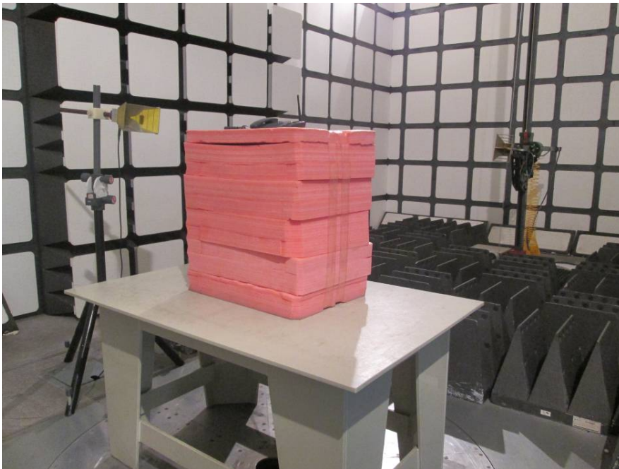
Radiated Emissions Test View (Above 1 GHz)
