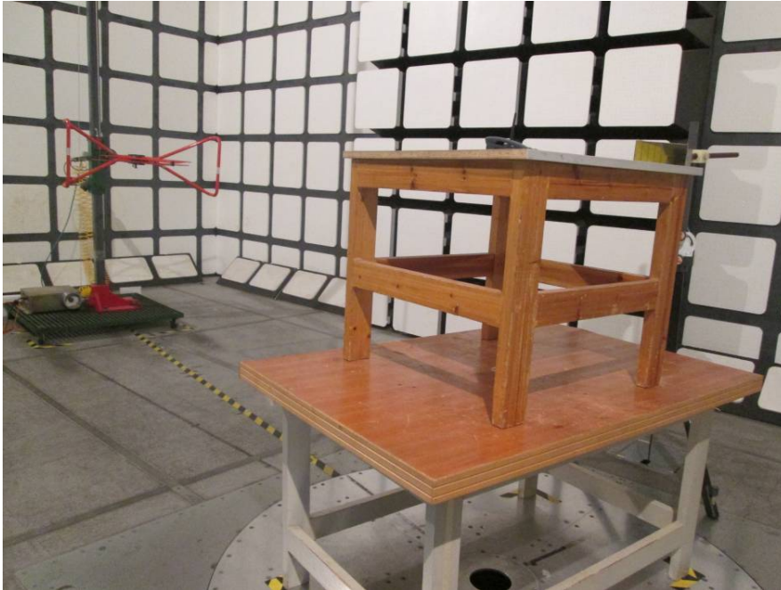
Radiated Emissions Test View (Below 1 GHz)
