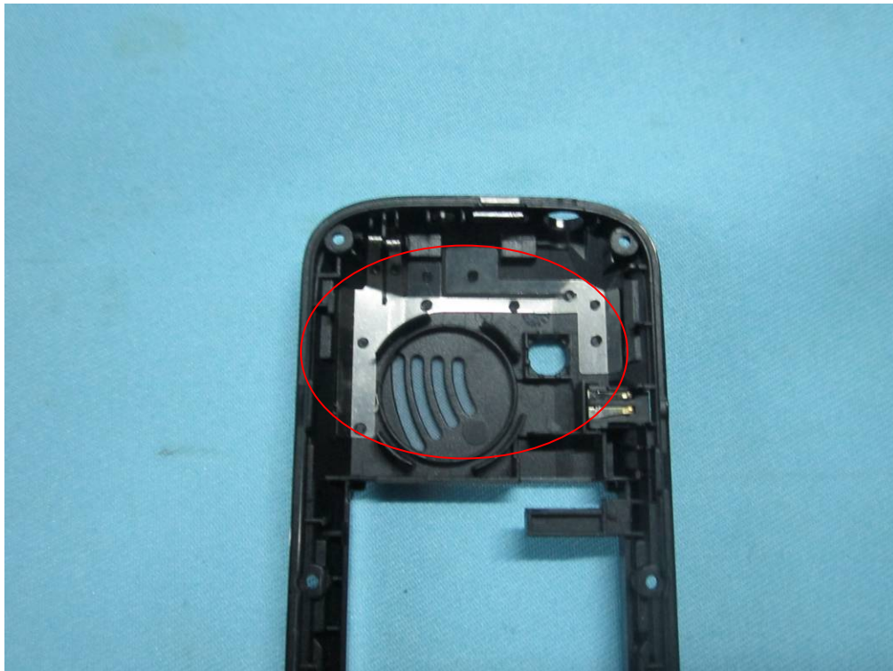
GSM Antenna View
