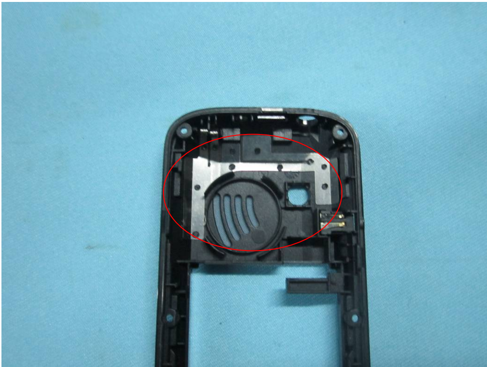
GSM Antenna View
