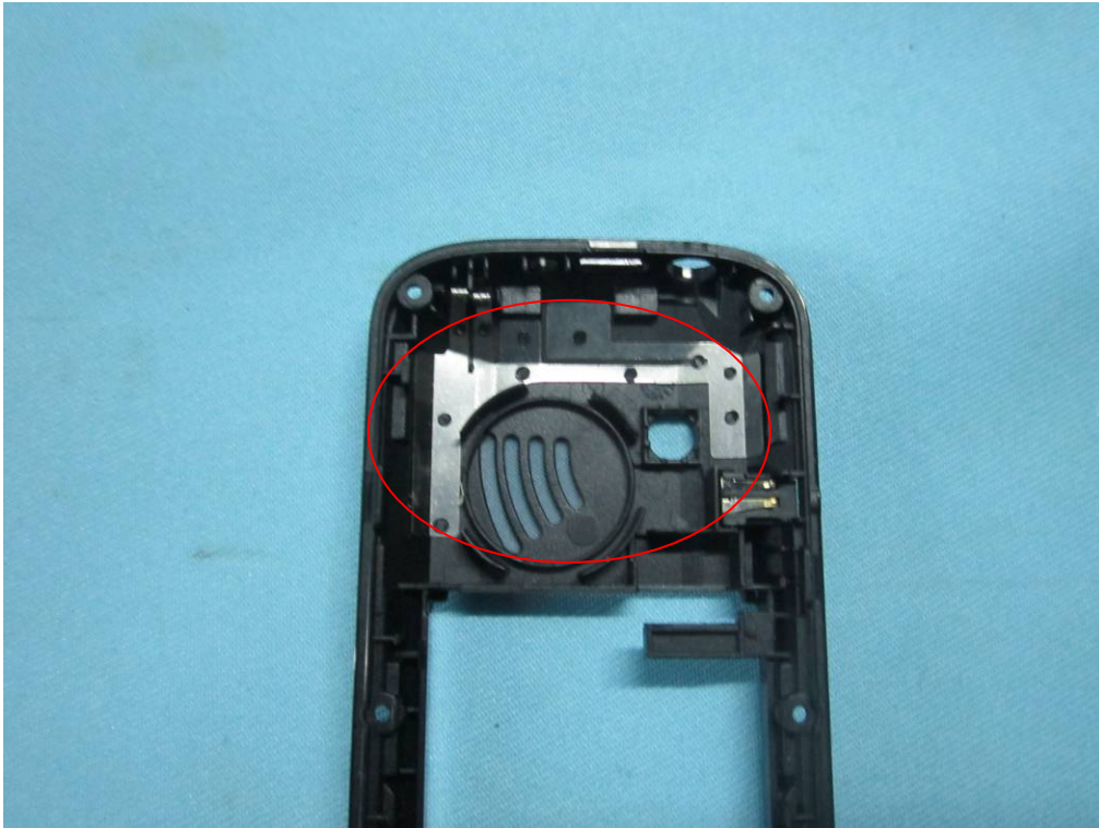
GSM Antenna View
