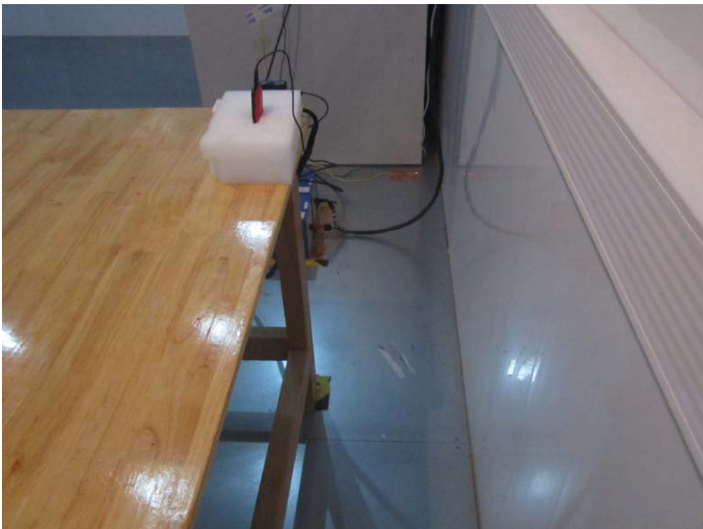
Conducted Emissions Test Setup Side View
