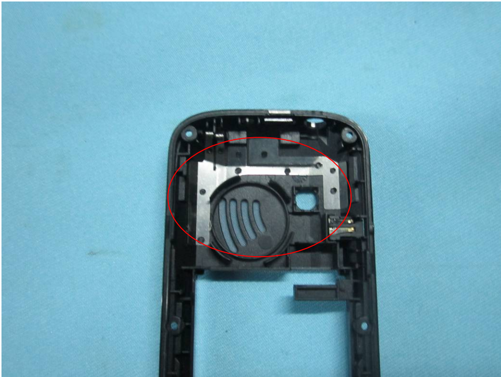
GSM Antenna View
