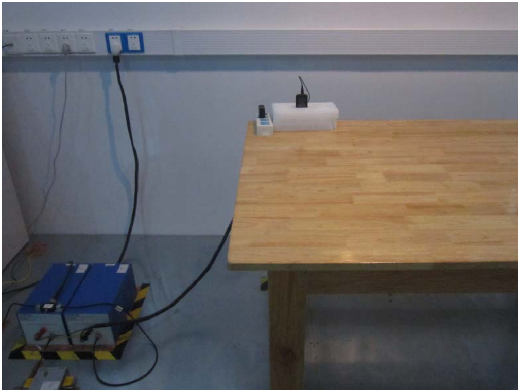
Conducted Emissions Test Setup Front View
