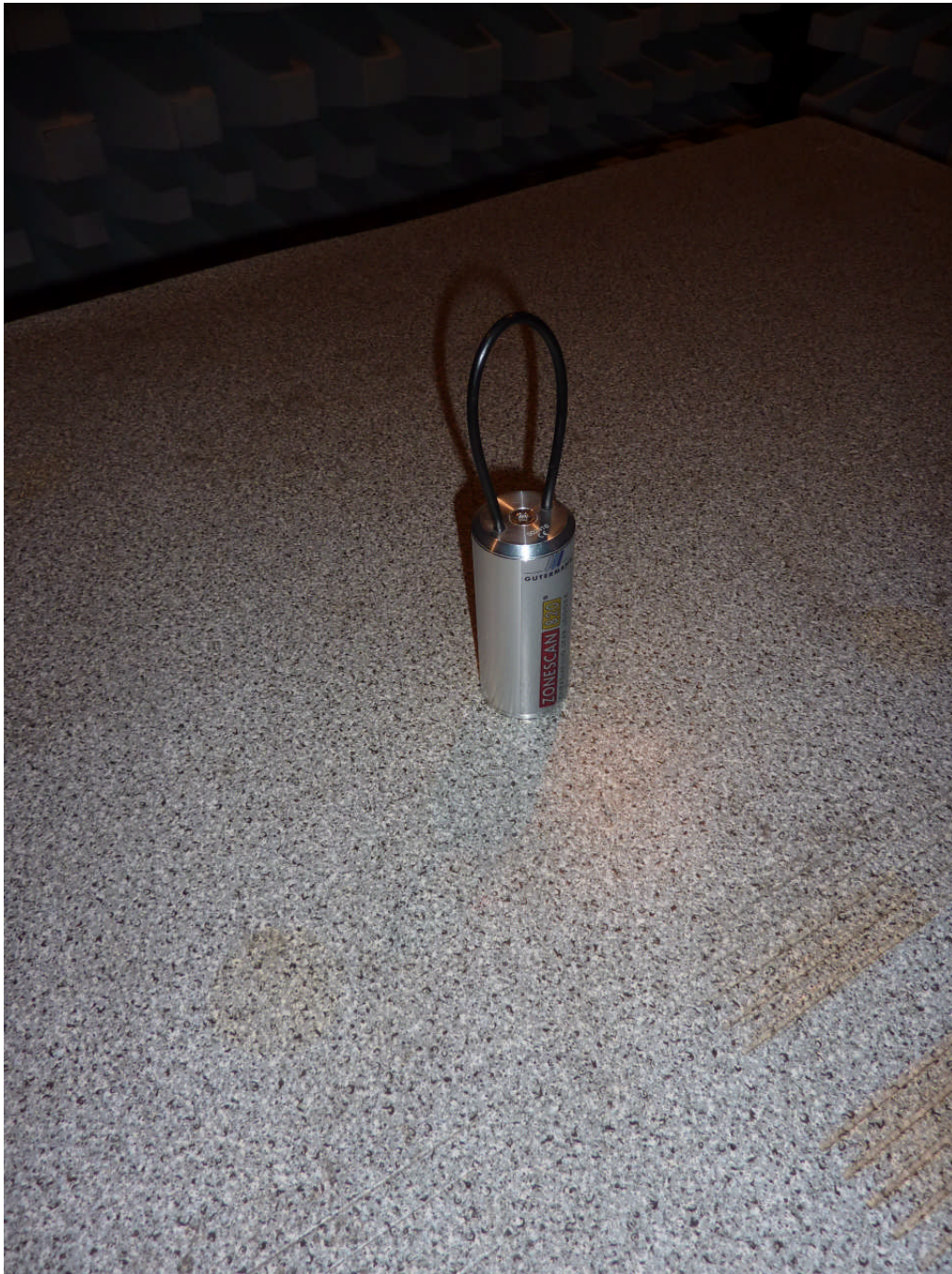
112414_1.JPG: Zonescan 820 Logger with internal antenna, test setup fully anechoic chamber
