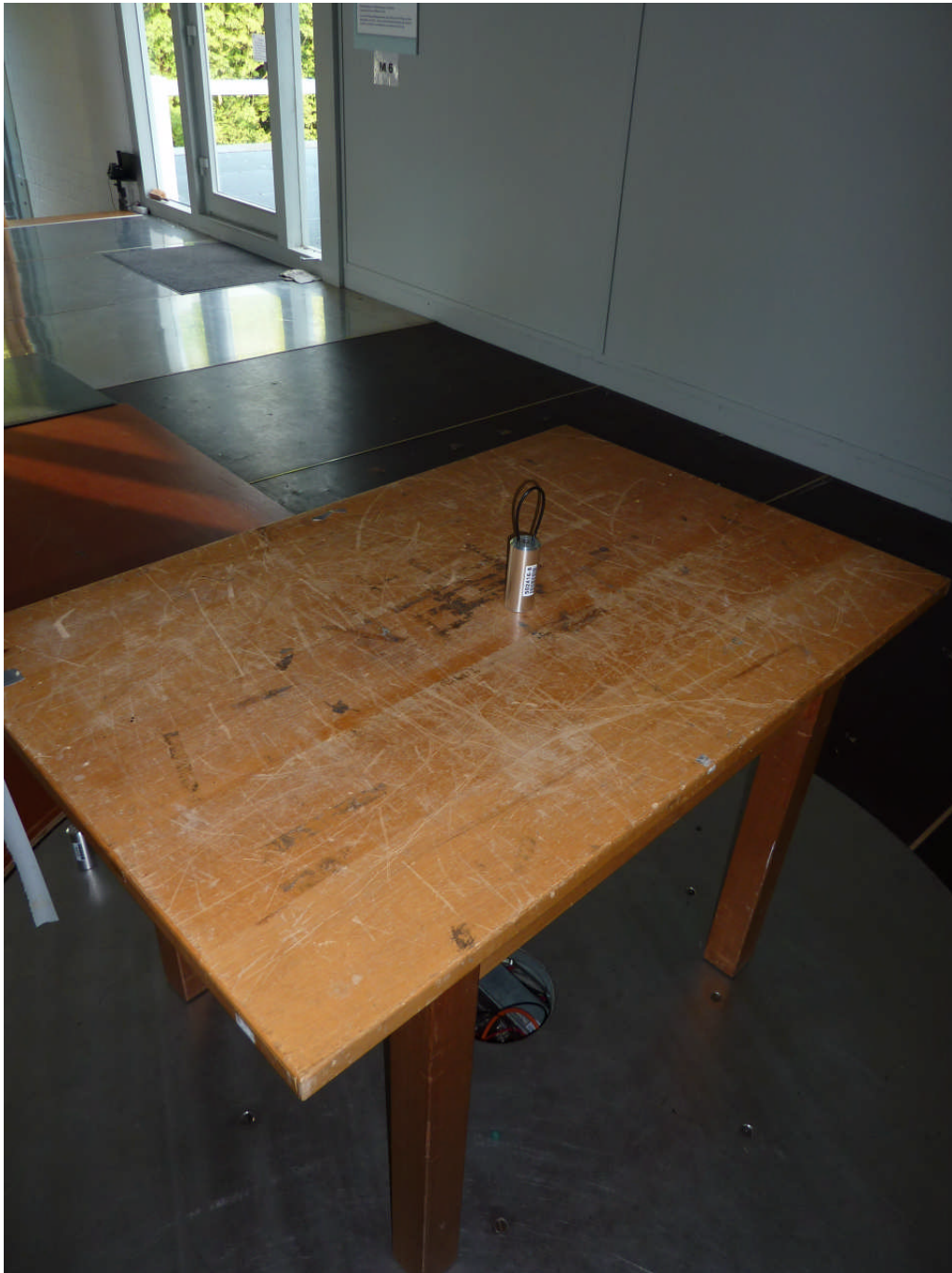
112414_9.JPG: Zonescan 820 Logger with internal antenna, test setup open area test site
