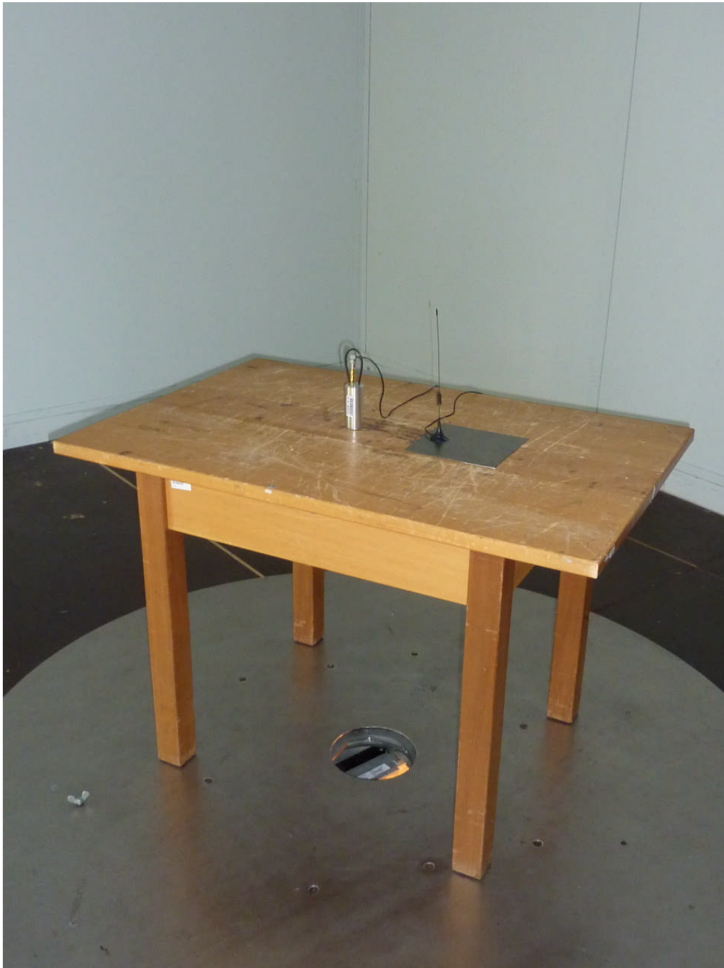
112414_10.JPG: Zonescan 820 Logger with external antenna, test setup open area test site
