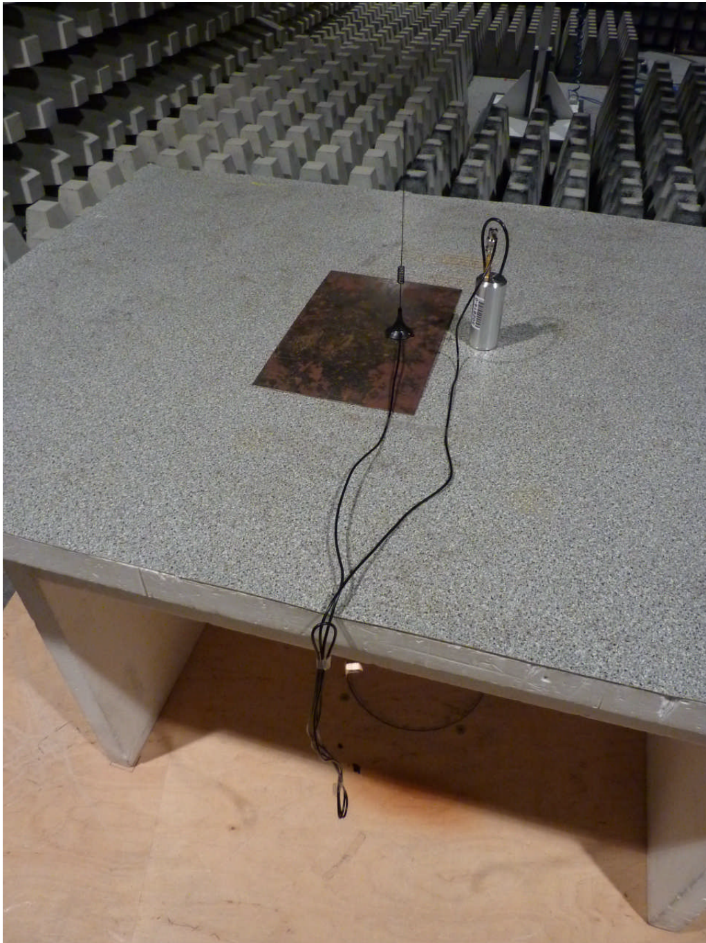
112414_4.JPG: Zonescan 820 Logger with external antenna, test setup fully anechoic chamber
