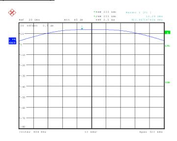
112414\_46.wmf: Maximum peak output power at the middle of the assigned frequency band (operation mode 2):
