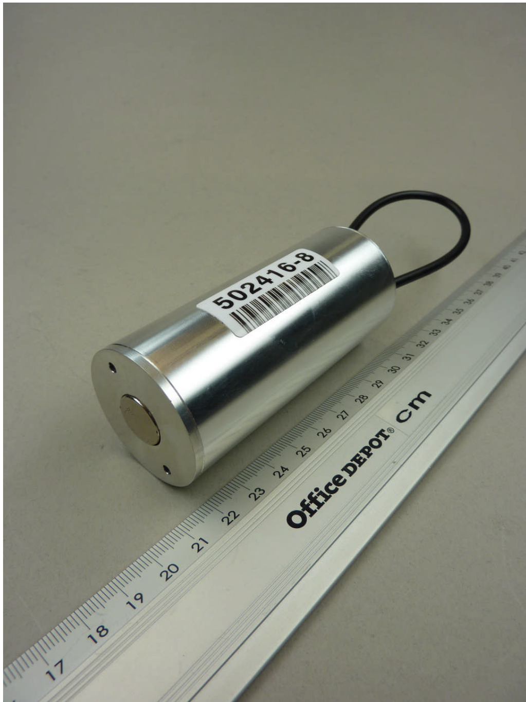
112414_i.JPG: Zonescan 820 Logger (with internal antenna), 3-D view 2
