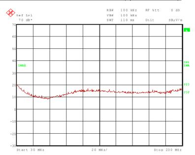
112416\_2.wmf: Spurious emissions from 30 MHz to 230 MHz (operation mode 1):
