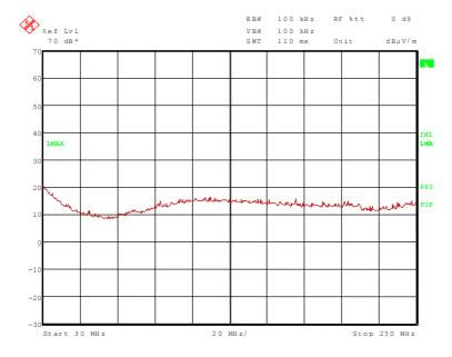
112416 6.wmf: Spurious emissions from 30 MHz to 230 MHz (operation mode 3):
