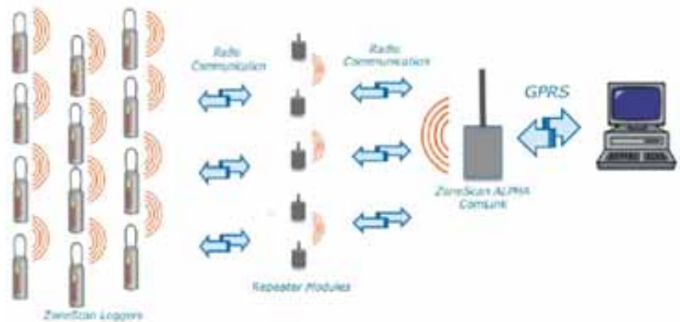
Figure 1 Functionality of logger, repeater and Alpha
