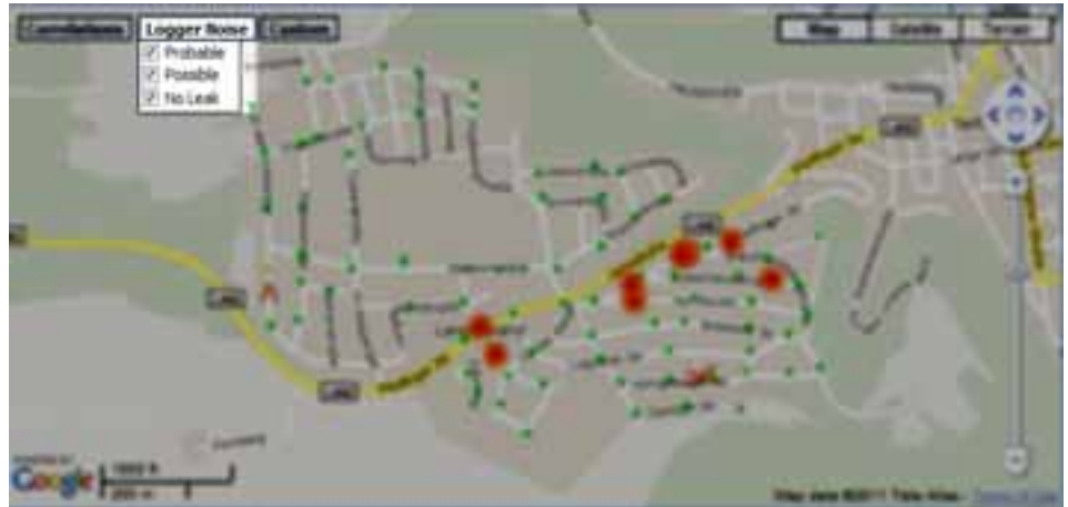
Figure: 2.8 Logger Noise Drop Down Menu
