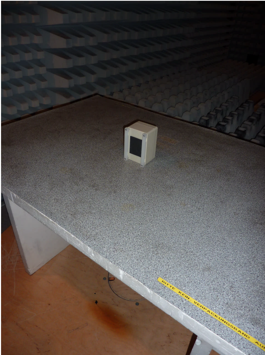
113573_6.JPG: ZONESCAN 820 ALPHA, test set-up fully anechoic chamber
