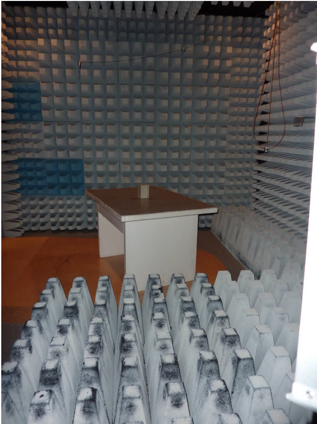
113573_4.JPG: ZONESCAN 820 ALPHA, test set-up fully anechoic chamber
