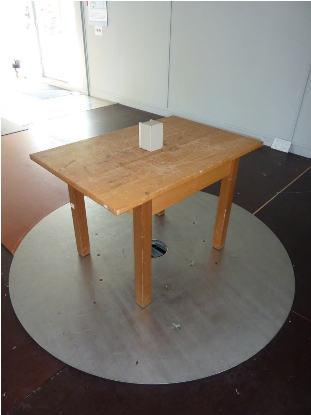
113573_7.JPG: ZONESCAN 820 ALPHA, test set-up open area test site
