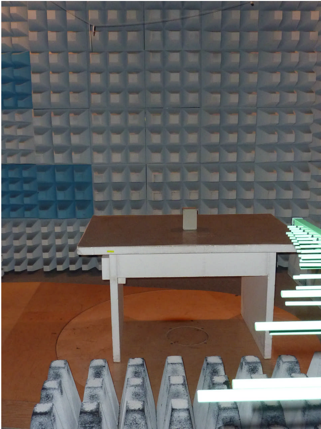
113573_2.JPG: ZONESCAN 820 ALPHA, test set-up fully anechoic chamber
