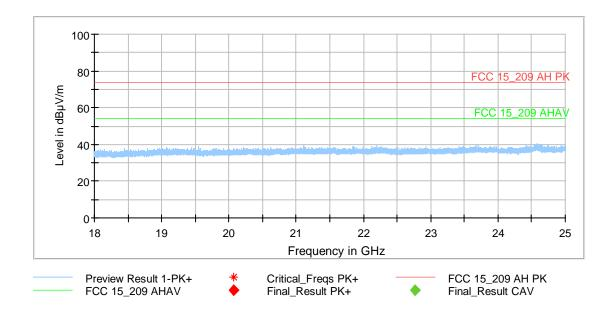
The following frequencies were found inside the restricted bands during the preliminary radiated emission test:
