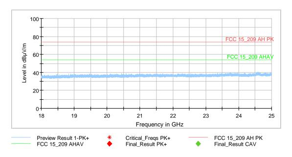
The following frequency was found inside the restricted bands during the preliminary radiated emission test.
