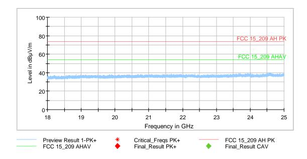
The following frequency was found inside the restricted bands during the preliminary radiated emission test:
