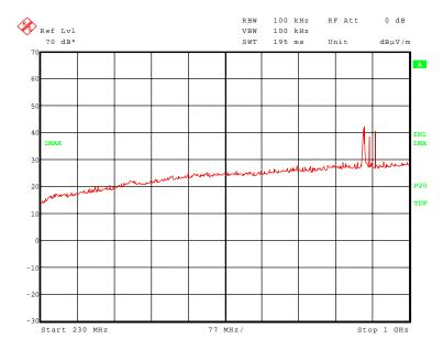
No emissions were found inside the restricted bands during the preliminary radiated emission test.
