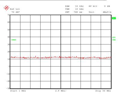
No significant frequencies above the noise floor of the system (max 30 dB $\mu$ V/m (measured with peak detector) at 3 m distance) were found during the preliminary radiated emission test, so no measurements were carried out on the outdoor test site.
