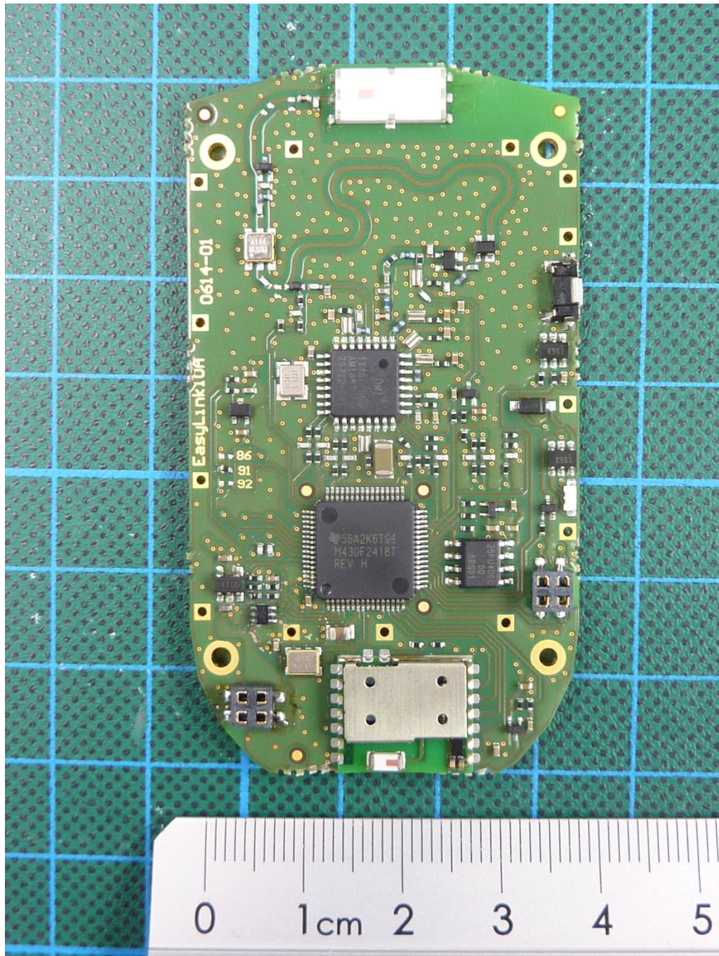
170032_13.JPG: EASYSCAN Link, PCB 2, top view, shielding removed
