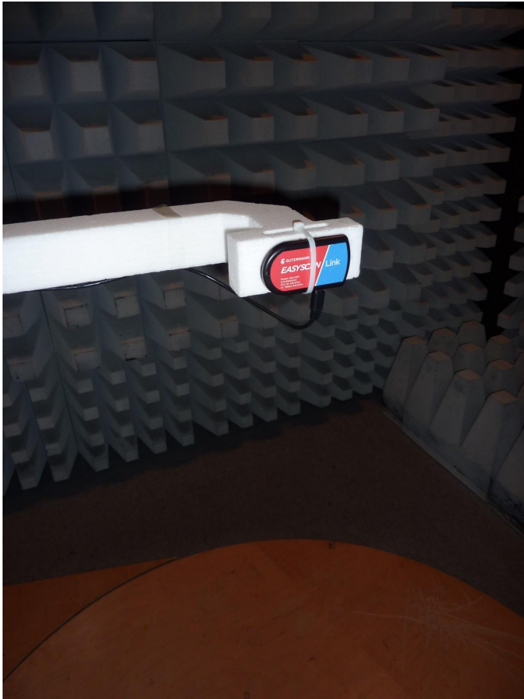
170032_a.JPG: EASYSCAN Link, test setup fully anechoic chamber
