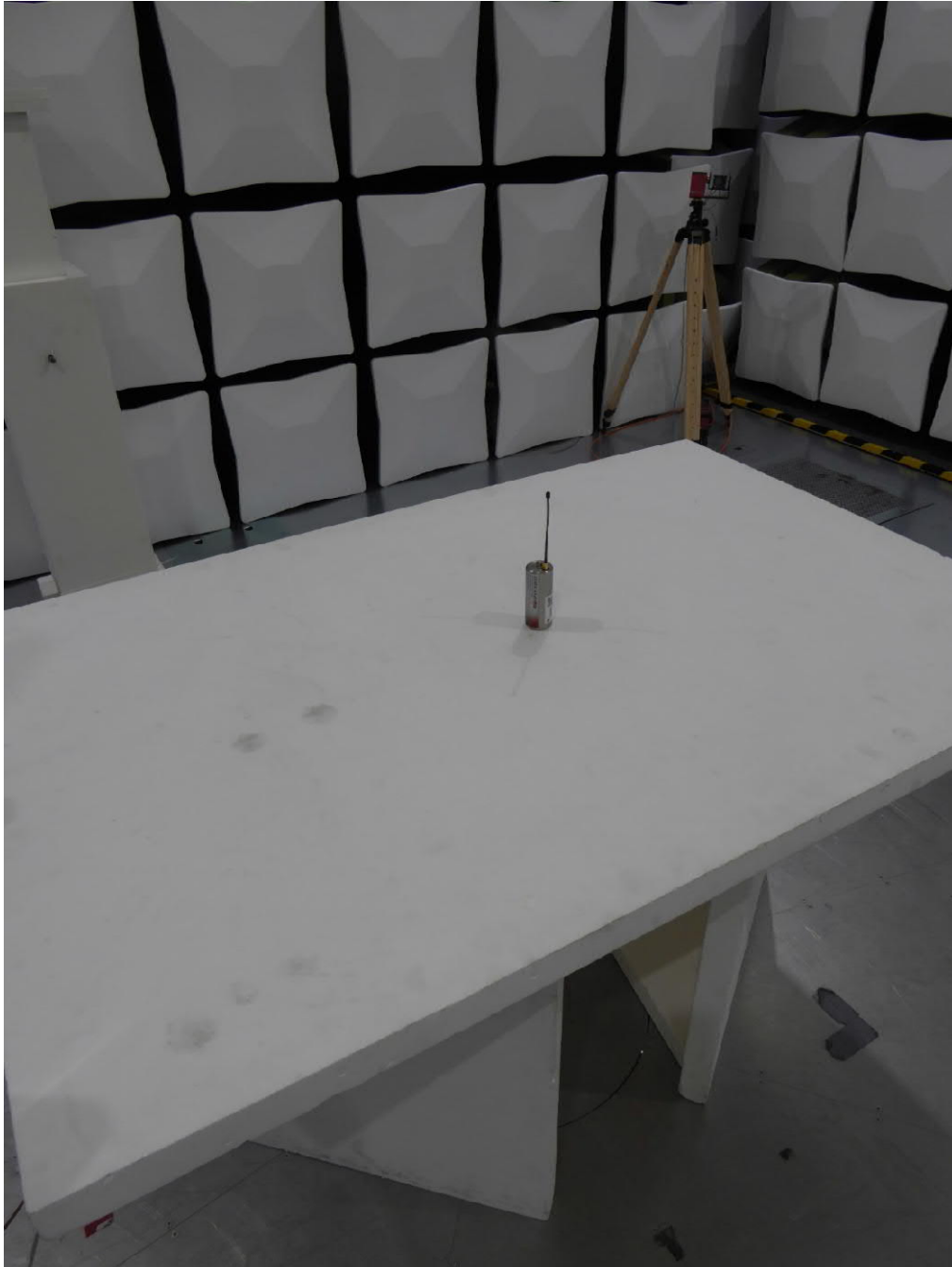
Setup 2 in SAC with ANT-ZS-NBIOT-90 Exemplary and worst case setup view (All ZS-NBIOT -Antennas and 3 orthogonal directions were tested)
