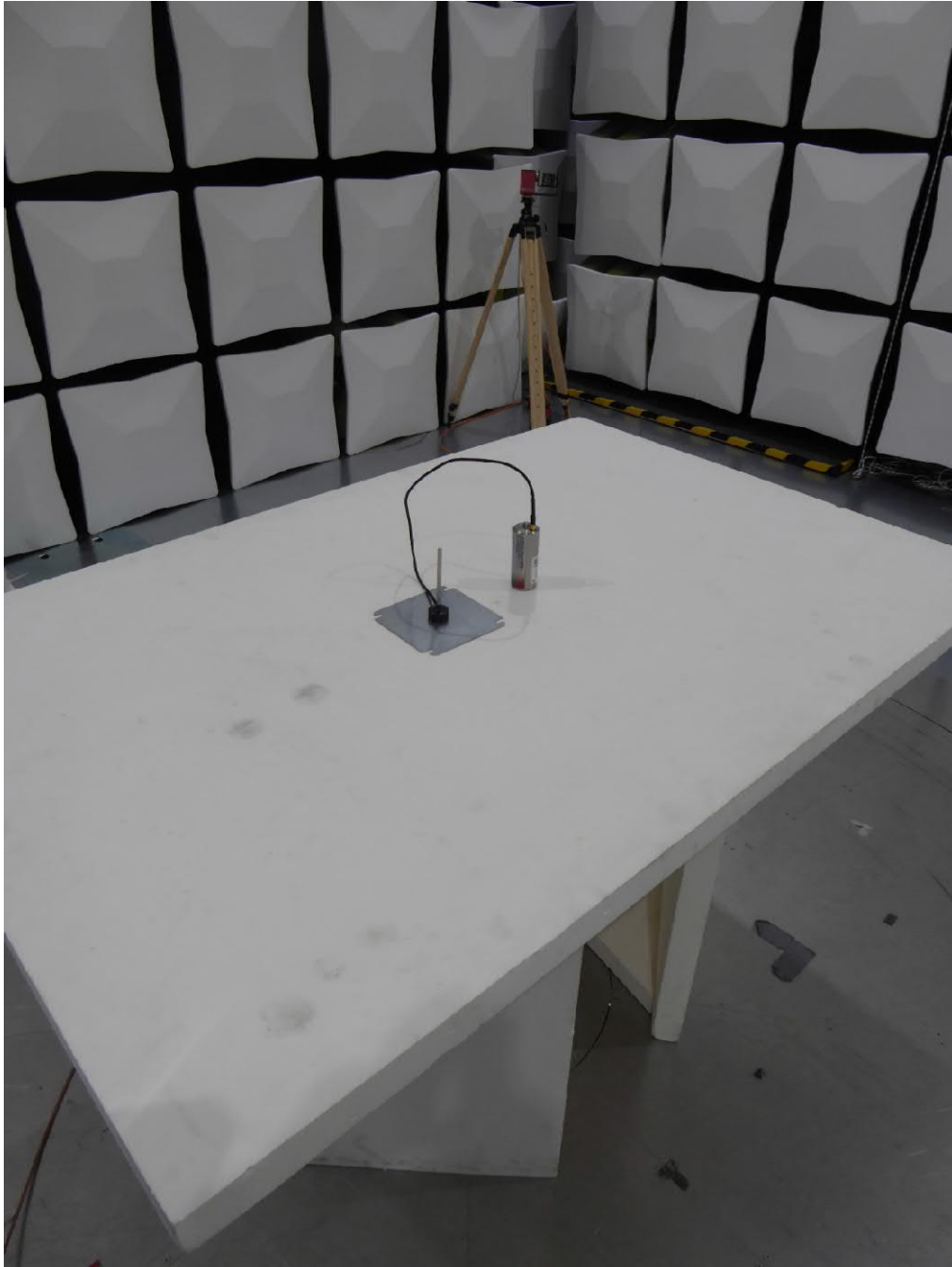
Setup 1 in SAC with ANT-BASE-15 and ANT-ROD-90 on 10 x10 cm groundplane Exemplary and worst case setup view (All ROD-Antennas and 3 orthogonal directions were tested)
