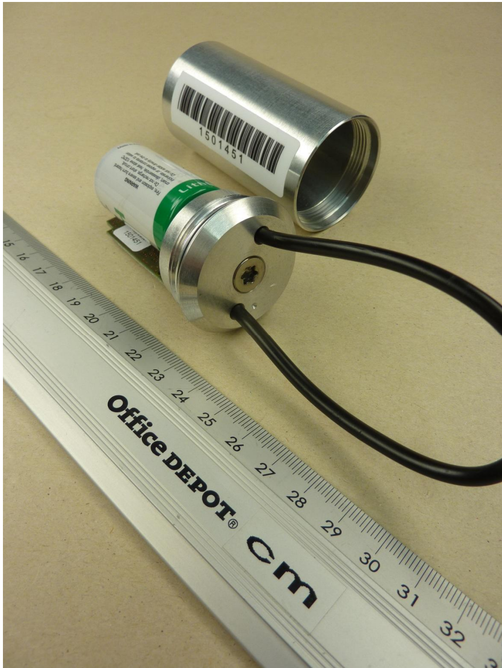
153494_R_U_5.JPG: ZONESCAN 820 Repeater, internal view 2
