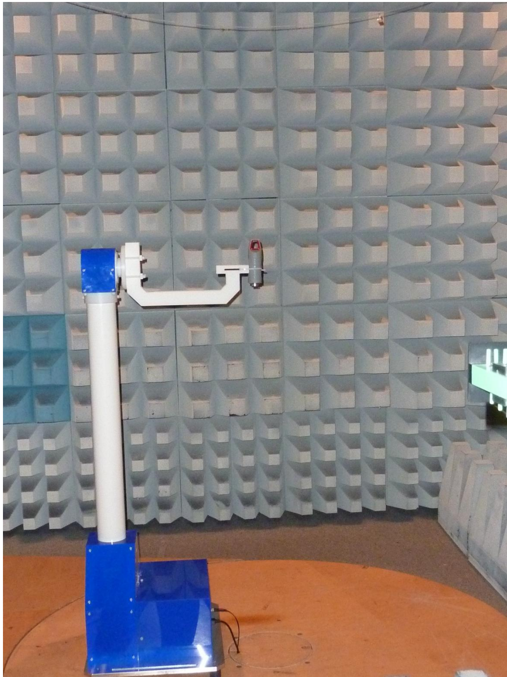
153494_E_U_I.JPG: EASYSCAN SENSOR, test setup fully anechoic chamber
