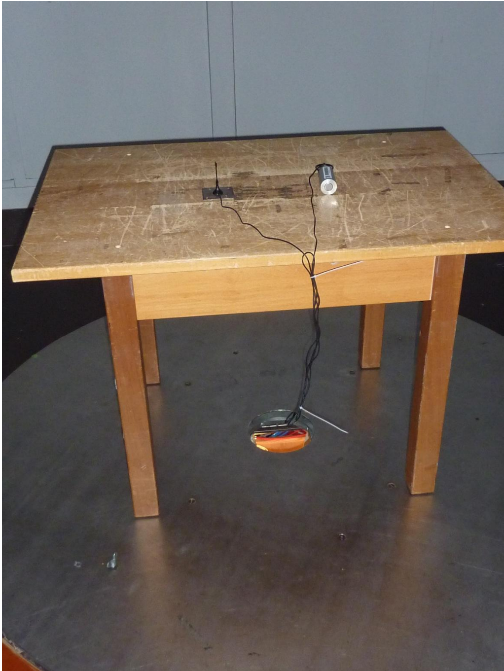
153494_X_U_H.JPG: ZONESCAN 820 Logger with external antenna, test setup fully open area test site
