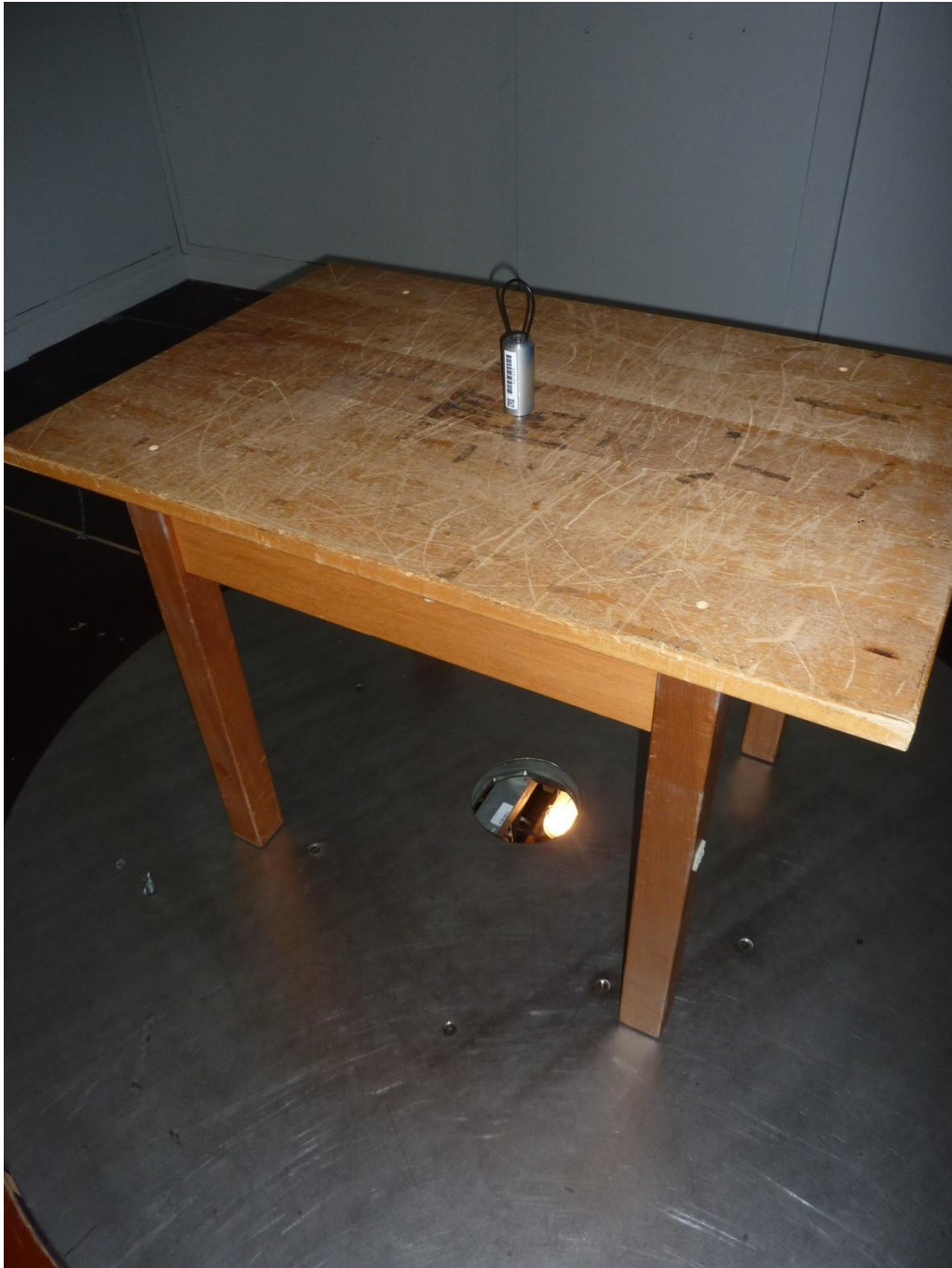
153494_I_U_J.JPG: ZONESCAN 820 Logger with integrated antenna, test setup fully open area test site
