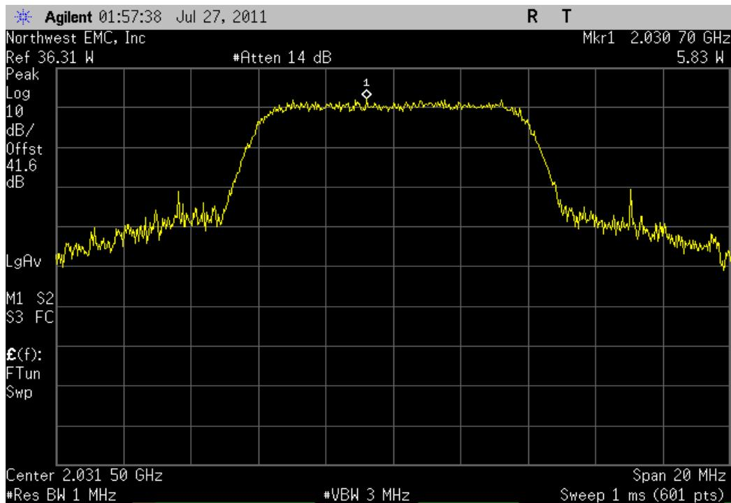
Port B, 16QAM, Mid Channel 2067.5 MHz
