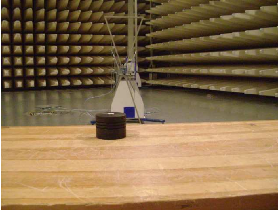
Photograph 1: Set-up for Spurious Emissions 30MHz – 1GHz
