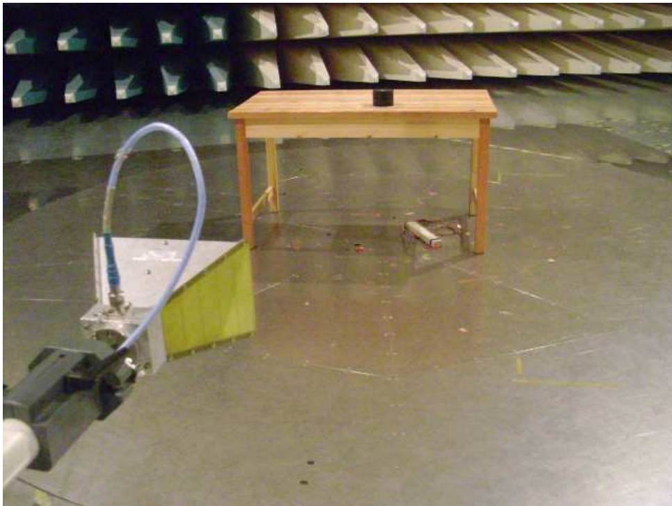
Photograph 2: Set-up for Spurious Emissions 1GHz – 12.75GHz
