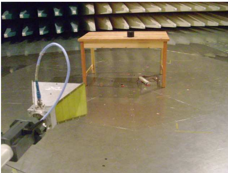
Photograph 2: Set-up for Spurious Emissions 1GHz – 12.75GHz
